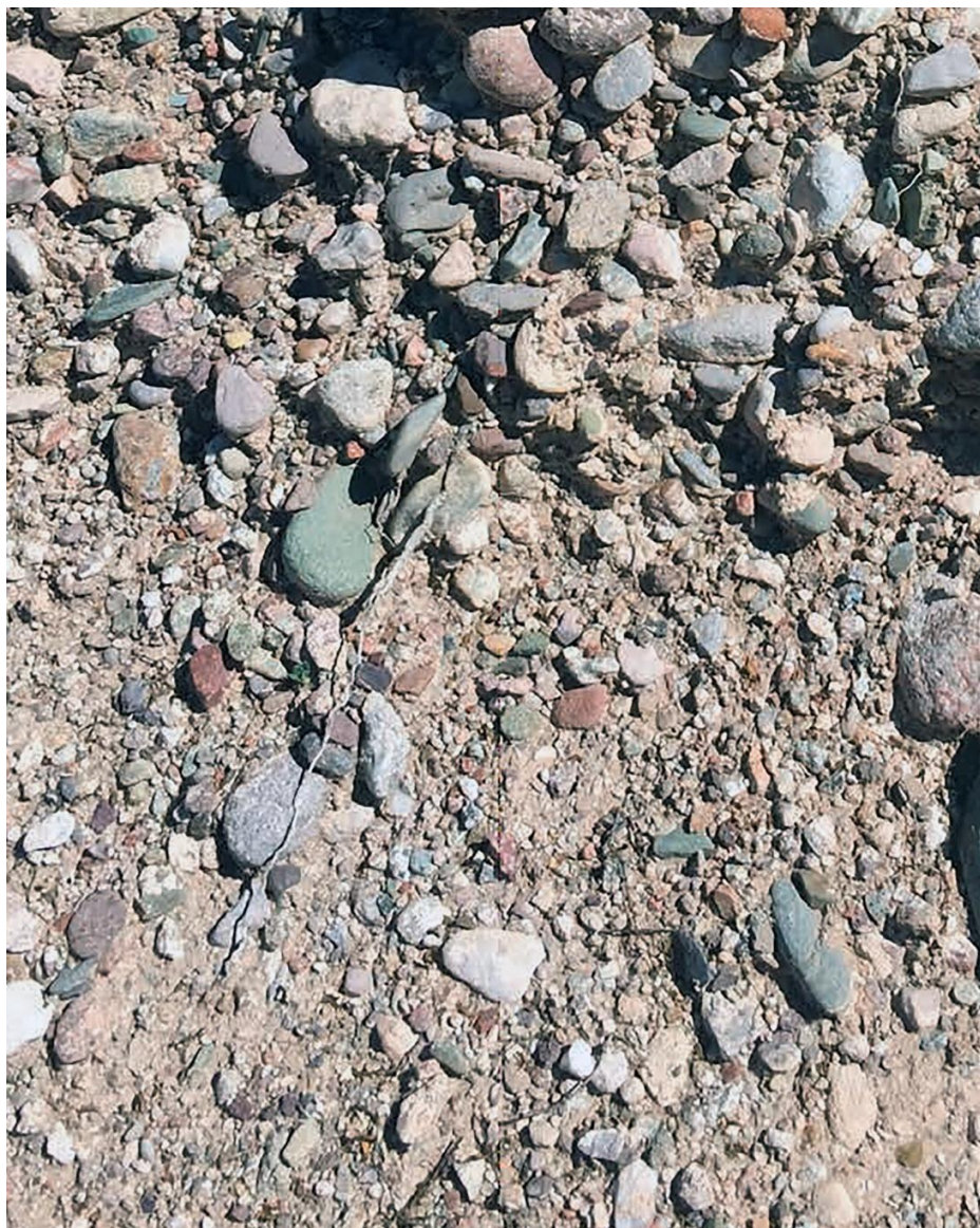
Figure 8 - Typical alluvial basin sediment fill; the interior of your aquifer may look like this (modified from Artiola et al., 2017).
