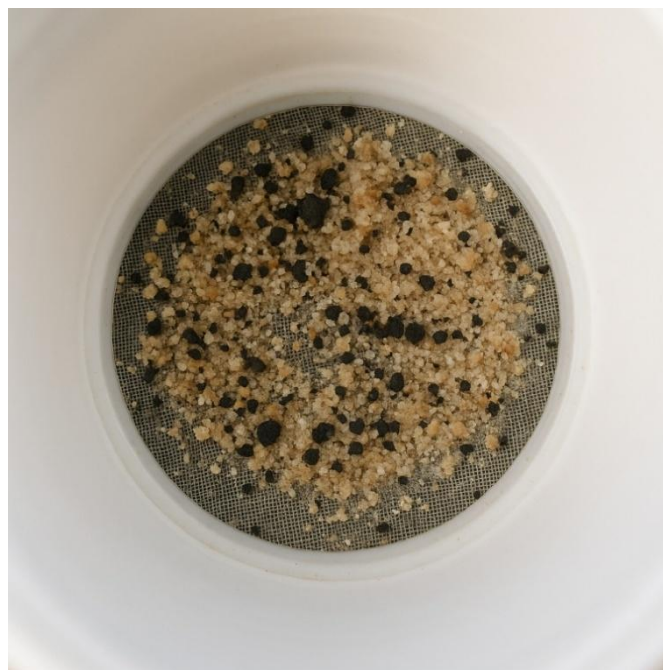
Figure 27 - Sand and precipitated manganese particles accumulated on the screen of an irrigation system (modified from Uhlman et al., 2012).
