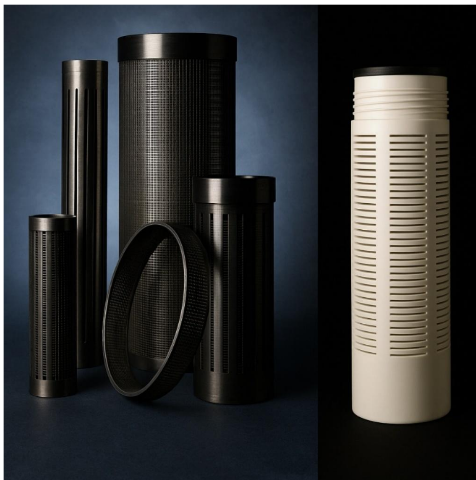
Figure 19 – Examples of well screens, showing continuous wire-wrapped metal screens (left) and a slotted PVC screen (right). Screens serve to filter out sediment. The screen slot size is ordered by the driller to fit the aquifer geology. (reprinted by permission of Johnson Screens, a Weatherford Company).
