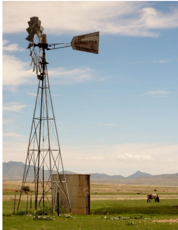
Figure 21 - Windmill-based well systems typically pump around 3 GPM, necessitating storage of water in tanks.
